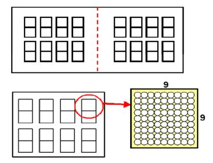
Figure 2.1: Array design for custom-made PCR-amplicon microarrays
